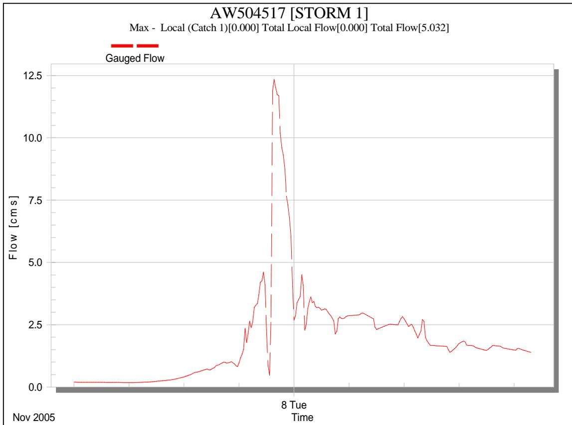
**Figure 2 Measured Hydrograph in First Creek Above the Waterfall**
