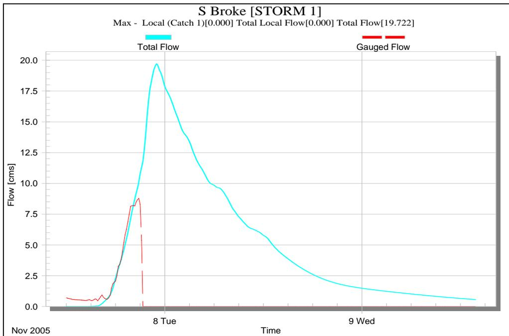
**Figure 1 Measured and Predicted Hydrograph in Fourth Creek at Stradbroke Road**
