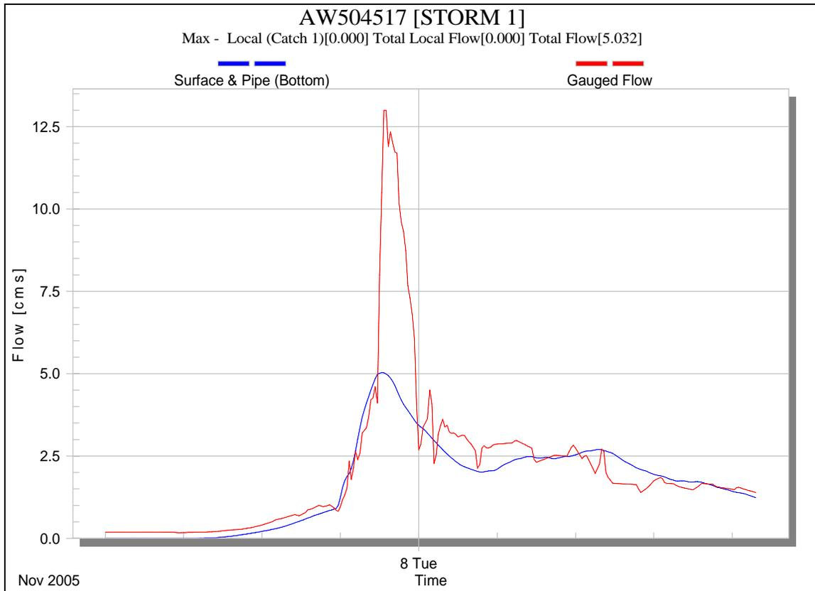
**Figure 5 Adjusted Hydrograph and Predicted Flow in Waterfall Gully**
