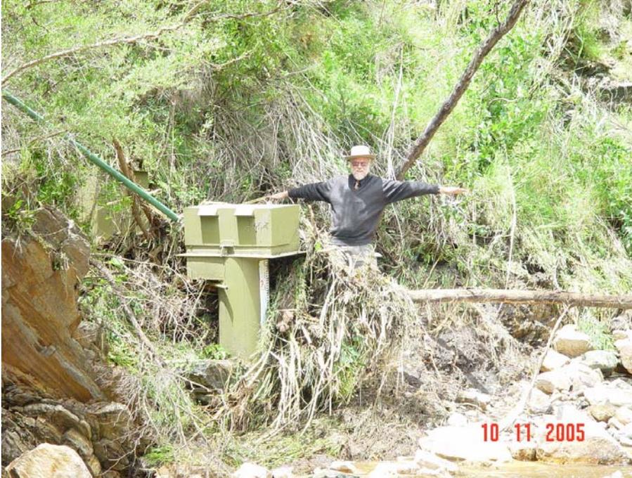
**Figure 3 First Creek Gauging Station Above the Waterfall - Author Showing Peak Water Level**
