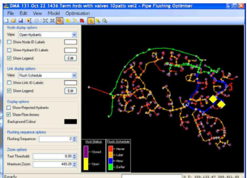
OptiFlush user interface showing solution layout
